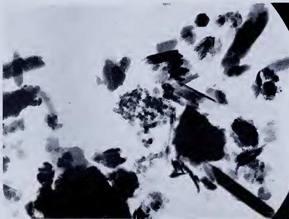
Figure 9.—Electron micrograph of white basal clay at Jarrahdale, showing kaolinite crystals, metahalloysite tubular crystals, and particles of amorphous gel. x 30,000.
